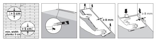
Measure the room to create a balanced layout. This will help you determine whether the first row needs to be cut. The first and last rows should not be less than 5 cm wide.
