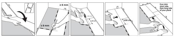
Always make sure that the short end joints are staggered by a minimum of 30 cm or three click elements when you start the next row. Use the leftover piece from the previous row as the first piece of the next row, provided that this piece is at least 30 cm long. In order to find a connection with the locking tabs of the previous row, it may be necessary to cut off an extra part of the leftover piece.
